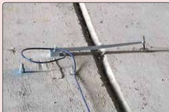
• Model 4420-3 Low Profile Crackmeter for measurements in the "Z" direction.
