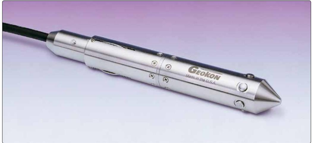
• Model 5000 Borehole Deformation Gage.
