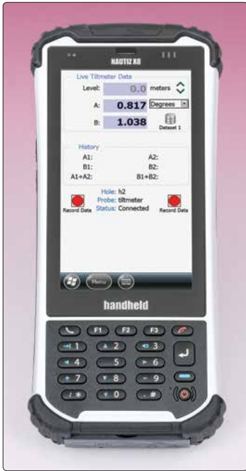
● Model FPC-2 Field PC showing a Live Tiltmeter Data reading screen shot.
