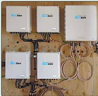
• Four Model 8032 Multiplexers connected to a Micro-1000 Datalogger.
