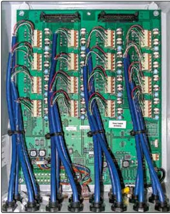
● Model 8032 16 Channel Multiplexer showing internal sensor connections.\*
