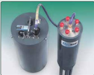
● Model 8600-3 Datalogger and Model 1150 (A-3) Extensometer (right).
