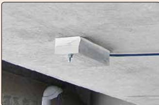
• Model ST-350, with cover, on girder.
